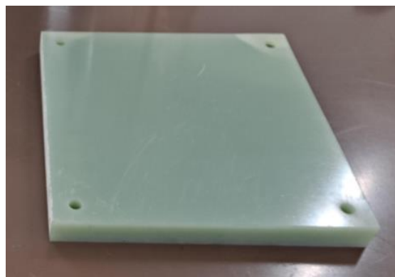
Figure 7.7 FR4 board blank ready for CNC machining of the profile of figure 7.6
