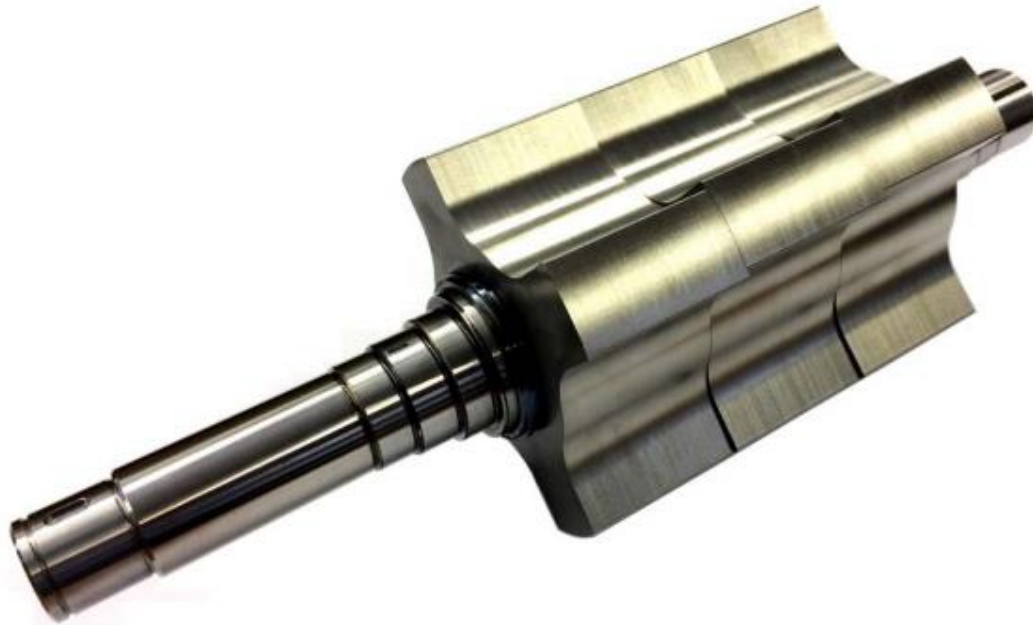
Figure 2.15 4 pole salient pole rotor for high speed operation with 3-stage step-skew (Source: [54])
