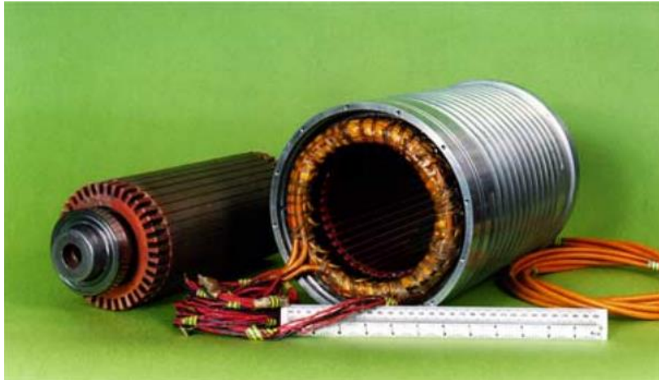
Figure 2.10 Components of a 26 kW induction machine producing 120 Nm at a base-speed of 2020 rpm (Source: [33])
