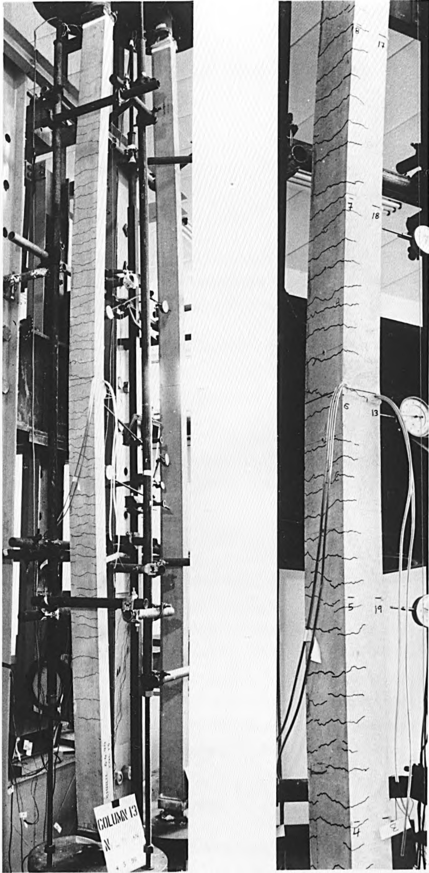
Fig.6.11 Typical crack pattern (C13).
