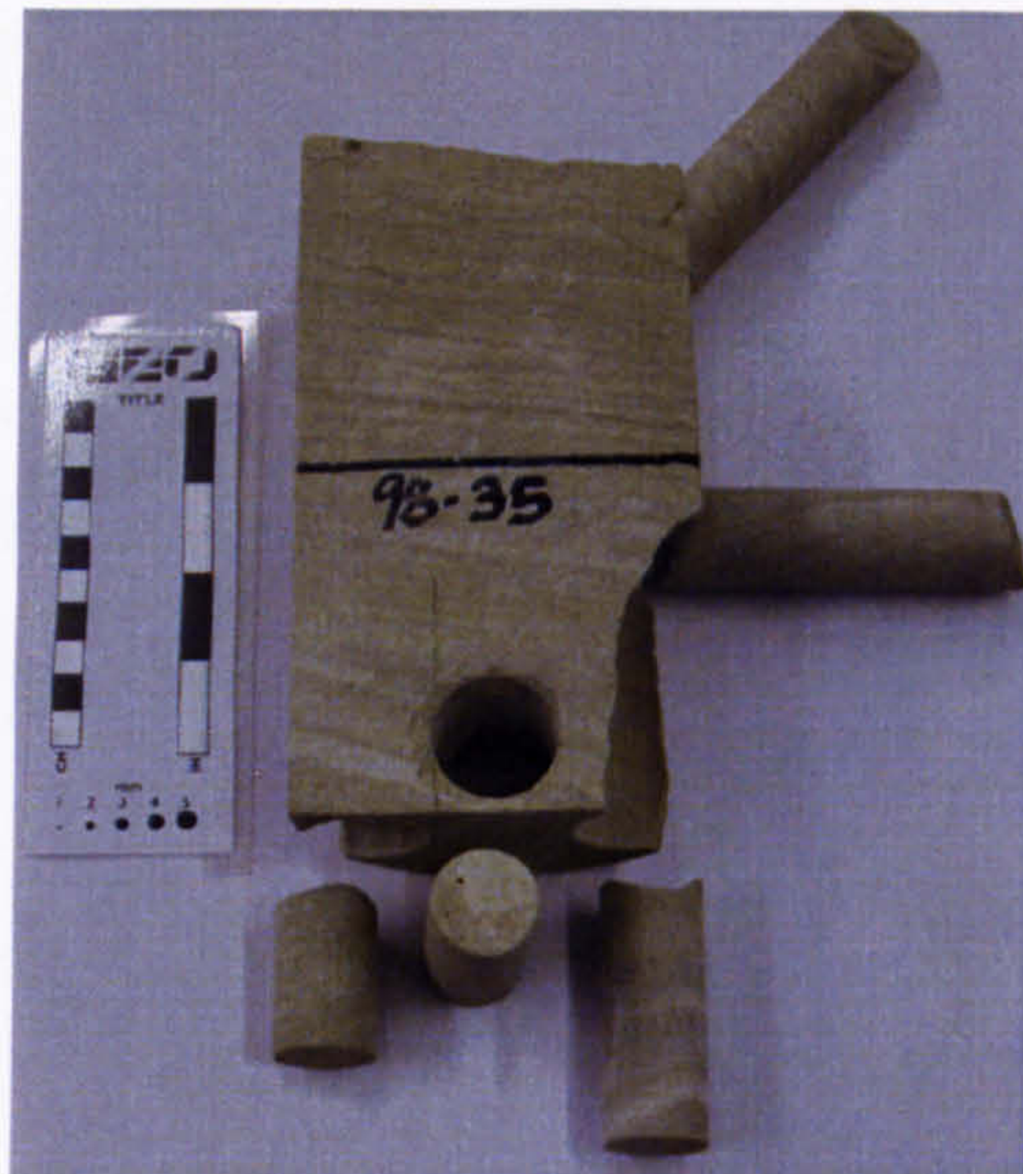
Figure 2.15: Half-core colour photograph of a typical Clair sandstone, with the four cores removed prior to ultrasonic testing. Sample number 2198m (Y-core) from Well 206/8-8.
