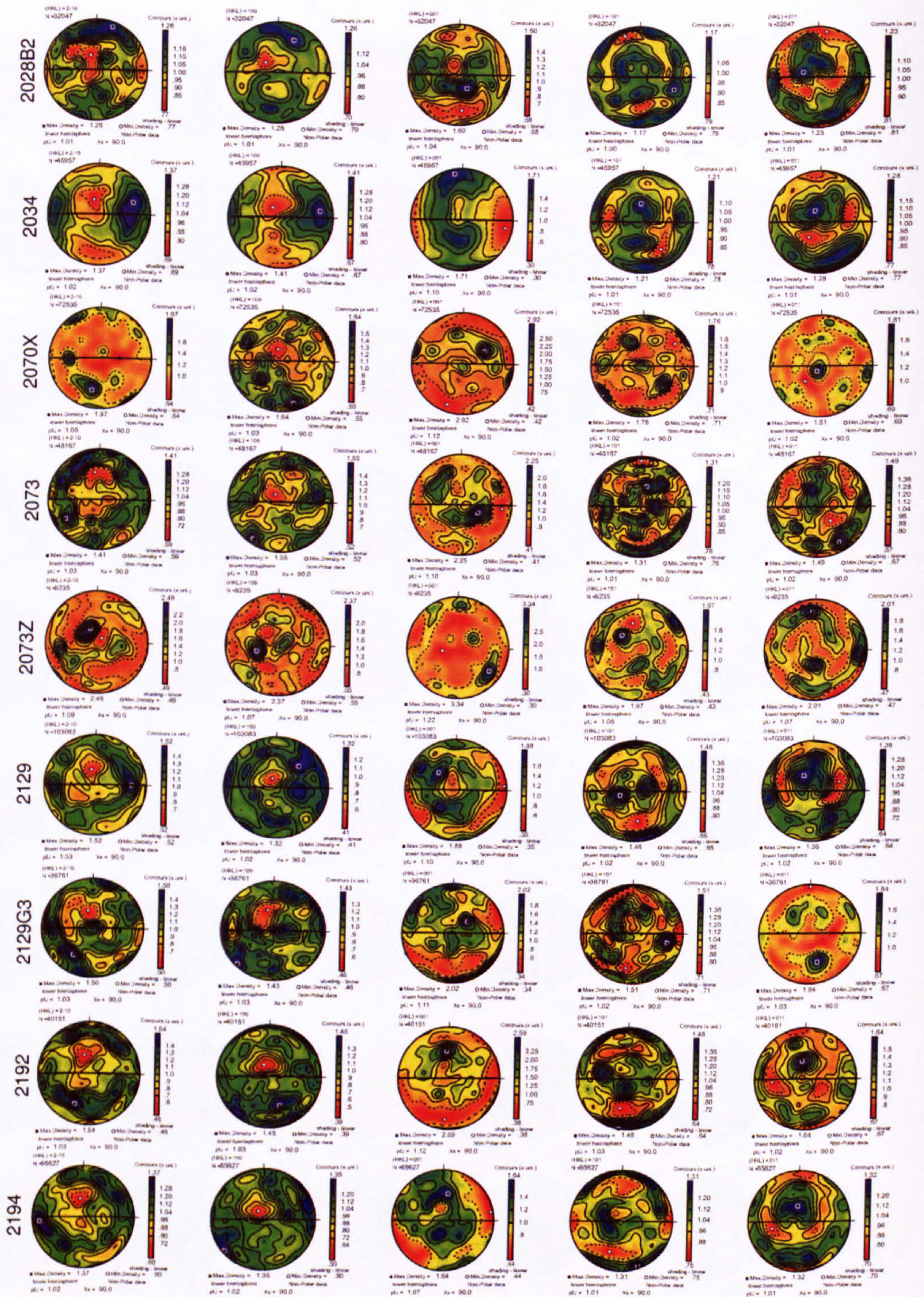
Figure E.3: Non-polar, lower hemisphere, crystallographic stereonets of quartz poles to lattice planes (2028m - 2194m). For an explanation of figure details see Figure (5.14).
