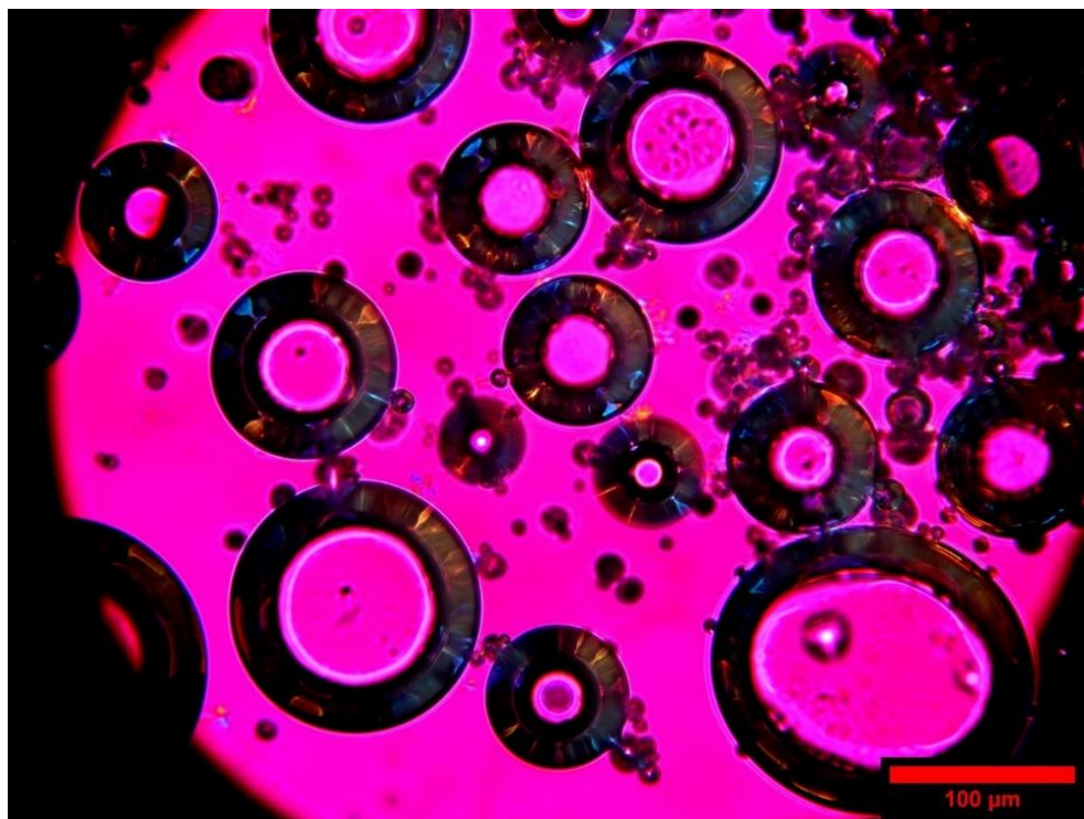
Figure A8. PLM image of a diluted 22F oleofoam with HOSO. Large air bubbles (diameter \sim 100 \mu\text{m} ) and small bubbles ( < 10 \mu\text{m} ) are visible. The image contrast was enhanced using a full-wave plate
