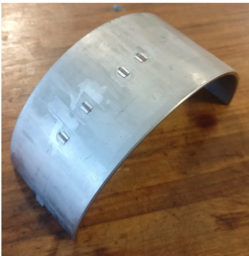
Figure 11.2: Photograph of bearing shell for BAXTER rig instrumented with longitudinal and shear ultrasonic transducers (left). Corresponding A-scan from a longitudinal bearing mounted sensor (right).
