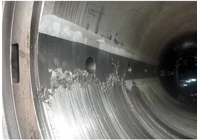
Figure 2.9: Photograph of wear in a stern tube bearing due to wiping [71].
