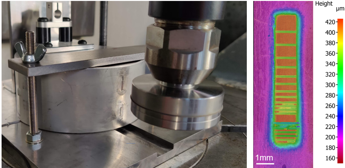
Figure 11.3: Photograph of bearing shell during array machining process (left). Surface profile of ultrasonic array taken using an Alicona InfiniteFocus SL (right).
