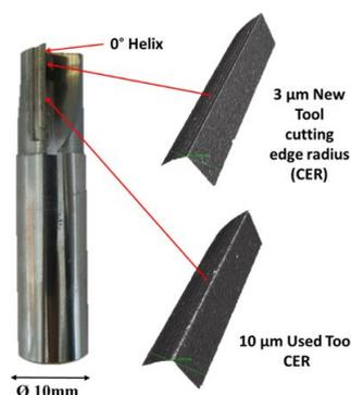
**Fig. 6.2.4.** Three flute Polycrystalline Diamond (PCD) Cutting Tool with Optical Edge Radius Measurements.
