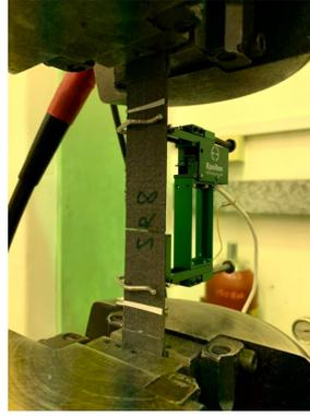
**Fig. 3.4.4.** Specimen breakage in tensile test with a fibre orientation of  $90^\circ$ .
