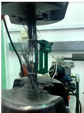
**Fig. 3.4.2.** Specimen breakage in tensile test with a fibre orientation of  $0^\circ$ .
