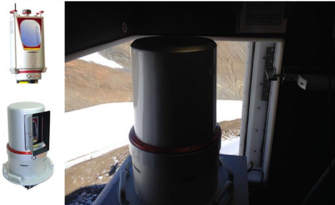
Fig. 3.3 Terrestrial laser scanner. This Riegl VZ-6000 unit has been permanently located near the summit of 'Im Hinterin Eis' near Hinteriesferner, Austria with a field of view over the glacier. The scanner is housed in a climate-controlled storage container and can be used to acquire repeated scans of the glacier, as demonstrated in Chapter 5. Images of scanner from riegl.com , main image from uibk.ac.at , by R. Sailer, Department of Geography, University of Innsbruck.
