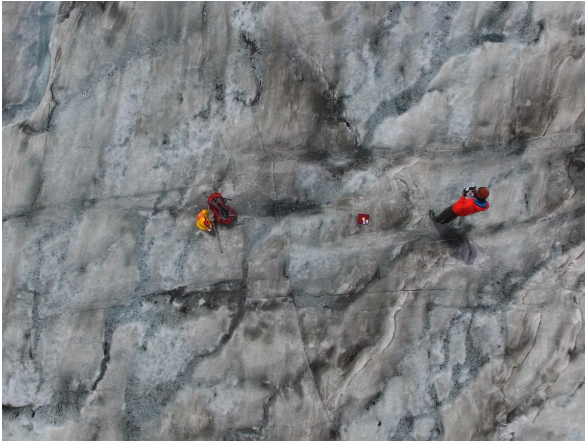
Fig. 3.2 Example of UAV photography. From an aerial vantage point, it is possible to capture the characteristics of a glacier surface over a broad area. This image also shows an example of a ground control point (red square with yellow dot and white number) used for georeferencing, along with the author demonstrating expert UAV piloting skills.
