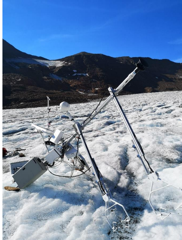
Fig. 2.5 Damaged sonic anemometer station on Hintereisferner, Austria. Differential ablation beneath the feet of the tripod caused it to fall, causing potentially expensive damage to the instruments and loss of hard-won data. Note the wind tower in the background is still vertical.
