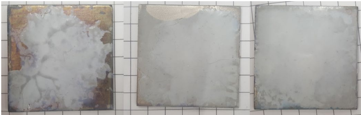
Figure 114: Optical images of Bioglass coating on Ti substrates – all samples are 3 x 3 cm
