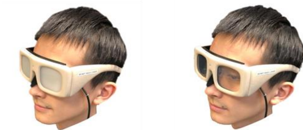
Figure 4.5. Side-by-side photos of occlusion spectacles in the open state (right) and close state (left).
