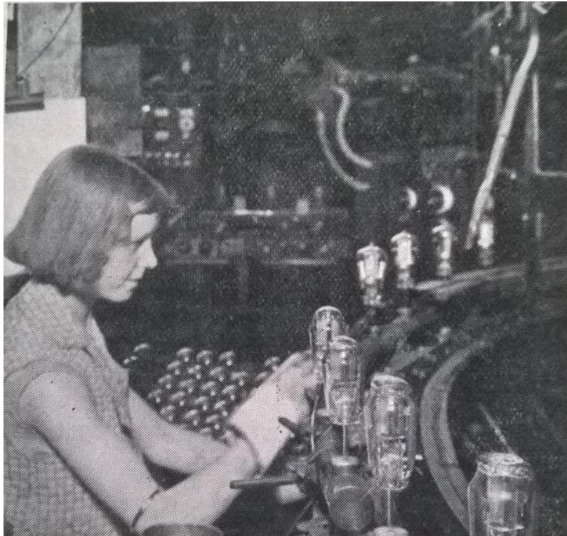
Figure 16 Pumping Machines at Cossor Valve Works 443
