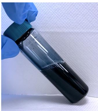
**Figure 3.5:** An example of a PEDOT:CS aqueous suspension displaying a clear dark blue-black colour, indicating the presence of conducting doped PEDOT.
