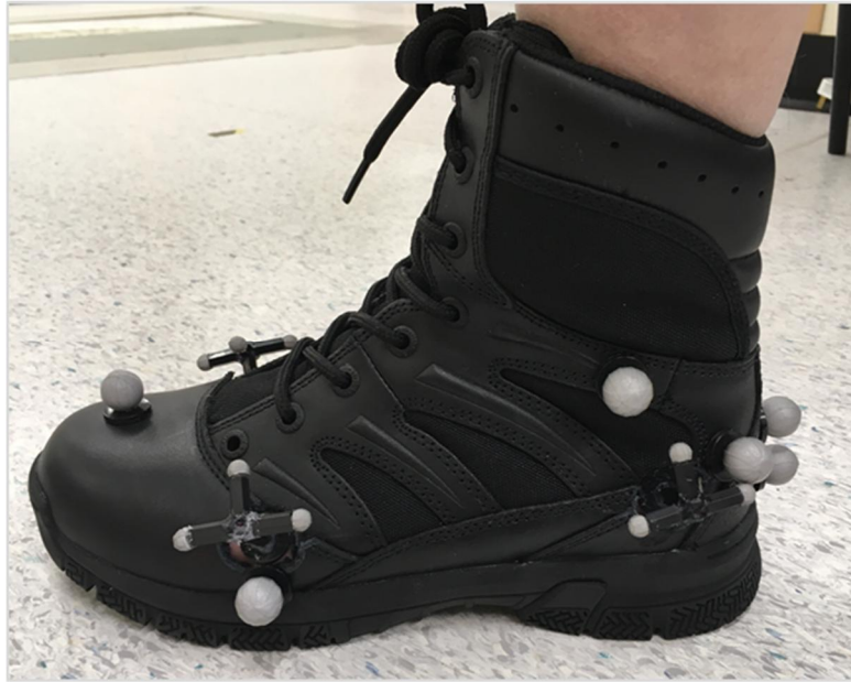
Figure 16: Pilot Military boot with foot and boot-mounted marker sets
