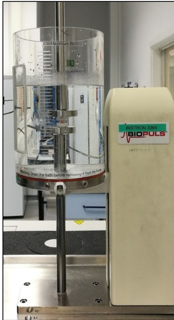
Figure 3.10: Specimen setup within Instron 3365 whilst immersed within a temperature-controlled Biobath.
