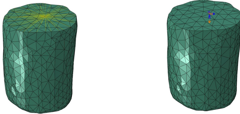
(i) Coupling constraint between master node and surface nodes. (ii) Displacement boundary condition applied to master node.
