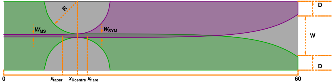
Figure 3.3: The copper artwork for each side of the antipodal Vivaldi antenna annotated with key design dimensions. It is to be driven by a connector on the left hand side launching to the purple microstrip section of width W_{MS} . The microstrip tapers to a section of symmetric microstrip before following an exponential flare from x_{flare} out to the nose of the antenna.
