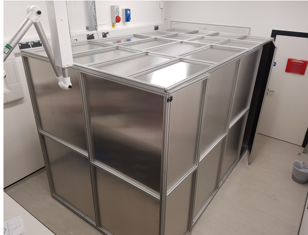
Figure 3.8: An external photograph of the completed anechoic chamber frame and sheet panels. When pushed shut, the doors seal against the adjacent panel with an overlapping section of aluminium sheet. Several bulkhead connectors were installed for cable lines into the chamber.
