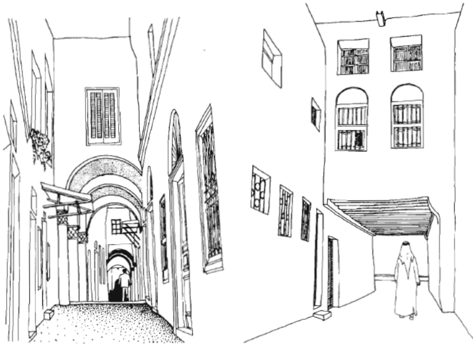
Figures 73A, 53B. “The Sabat – an air-tight structure bridging a public right of way is a concept designed to provide additional space for the building to which it is attached. It is used in most Islamic cities, acting as an element of unity. The local Urf in each city shapes its architectonics and thus contributes to the phenomenon of diversity” (Hakim, 2009, p. 117).
