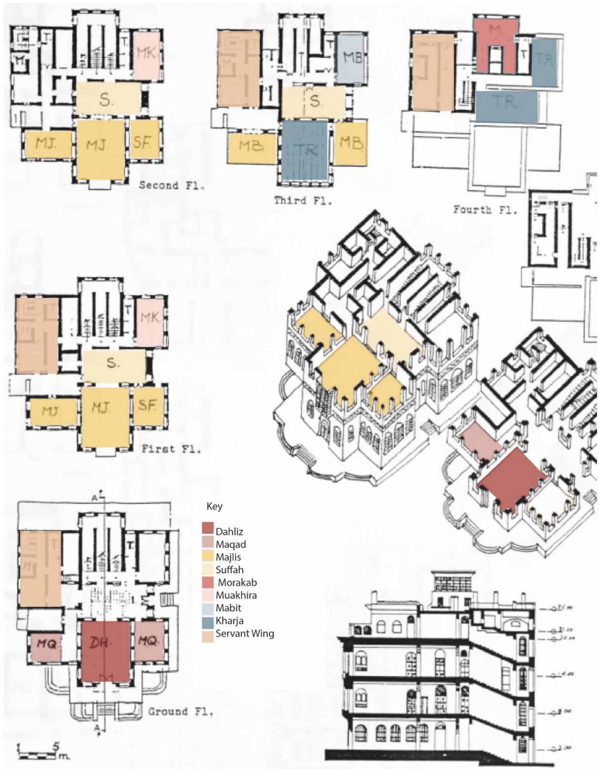
Figure 198: Nassif house floor plans, different colours were used to identify different spaces. Source: (Al-Lyaly, 1990, p. 51), edited by author.
