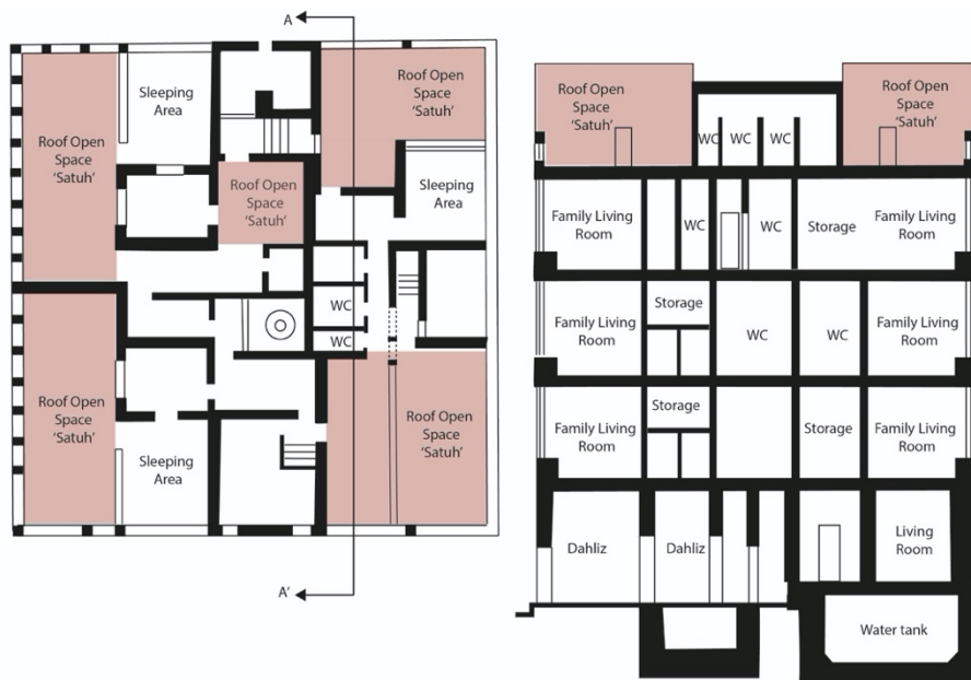
Figure 114: Most houses had more than one open roof, kharjah , which were situated in different levels on top of the house. Left, Al Hazazi House top floor. Source (Hariri & Sultan, 1995, p. 46) redrawn and edited by author.
