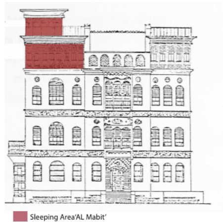
Figure 117: Nassif House showing the sleeping areas on different levels built into the roof open space. (Al-Lyaly, 1990, p. 128).
