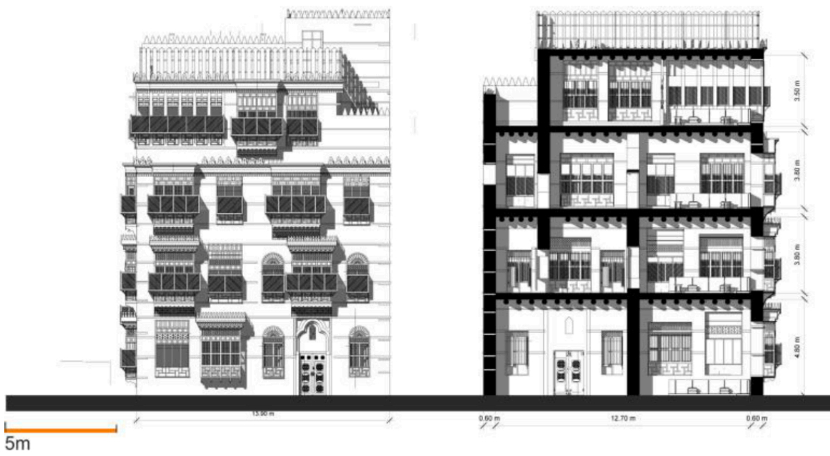
Figure 177: Left, west elevation of Bait Waqf Al Shafi. Right a section of the house. Source: (Khan, 2015, p. 183).
