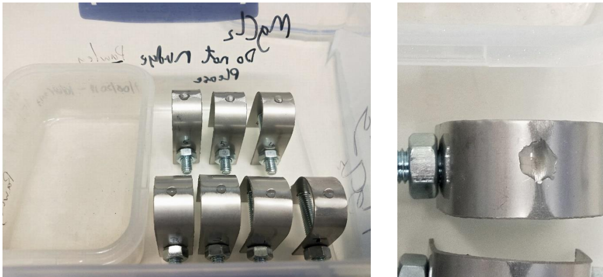
Figure 6.7 U-Bend stress tokens inside a humidity chamber alongside a saturates \text{MgCl}_2 solution. \text{MgCl}_2 droplets have been applied to the tokens.
