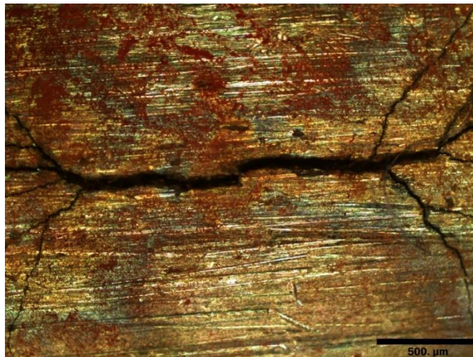
Figure 6.40 Showing the main central crack branching into multiple sub cracks.
