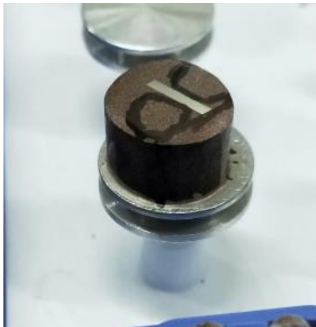
Figure 3.7 A Cylindrically mounted sample in ProbeMet, affixed to an SEM stub with silver DAG and with plastic ring clip covered with conductive ink.
