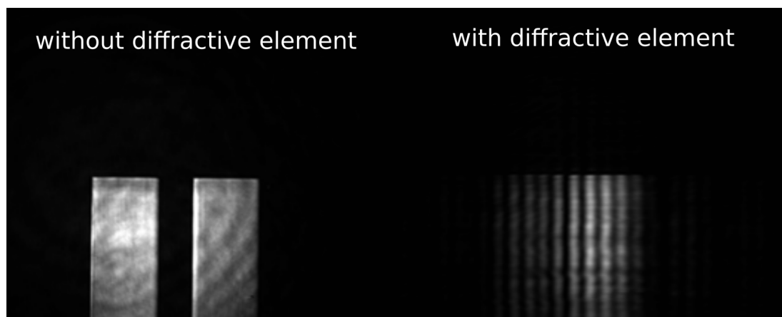
Figure 52: Raw images demonstrating sensing with a double slit as the diffractive element. On the left, two identical gratings are on resonance and are imaged. On the right, a double slit is aligned with the same gratings such that the light from each grating falls onto one slit only, thereby being able to interfere in the camera plane. The method is based on the well-known Young’s slit interference experiment. The images are meant to illustrate the working principle only.
