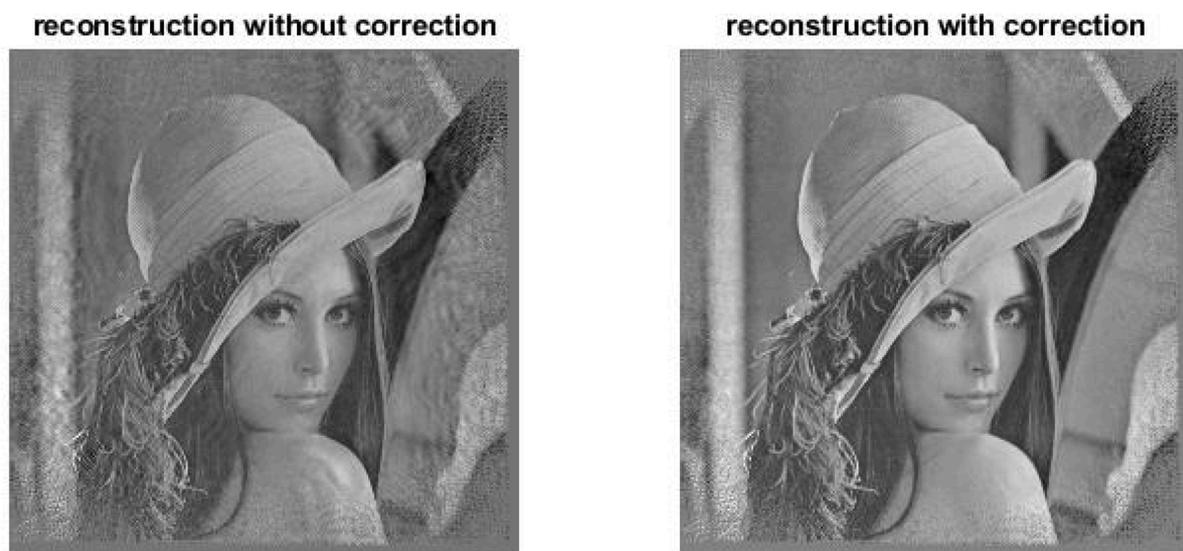
Figure 80: The phase reconstruction result with non-linear test data with and without detector correction. After the correction, the reconstruction shows better contrast, and the blurs in the left image have been removed when compared to the image on the right.
