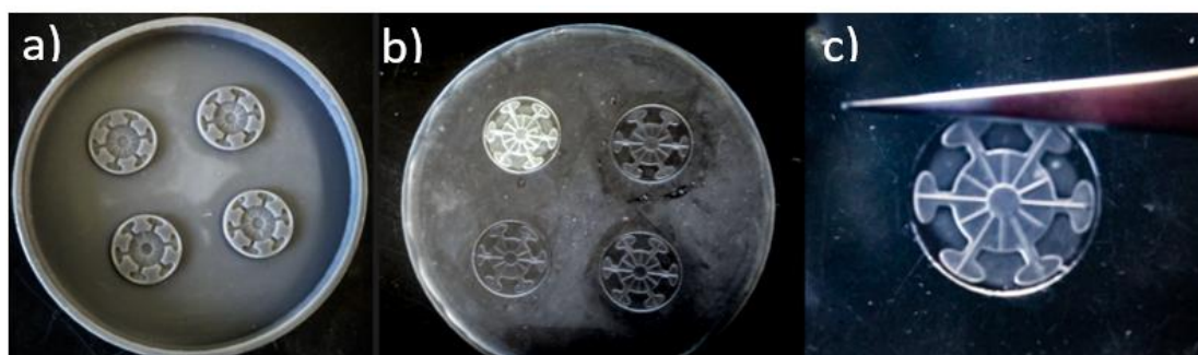
Figure 3.12 a) 3D printed moulds for flat scaffolds, b) silicone moulds (soft stereolithography) c) PGS-M scaffold
