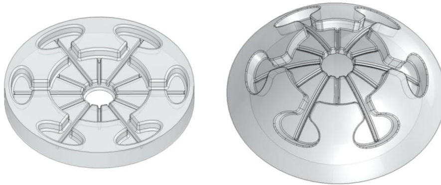
Figure 3.3 Flat (left) and dome shape (right) scaffolds with in-built artificial cell niches moulded in Solidworks 2019. Scaffolds have 1 mm of thickness and 15 mm diameter.
