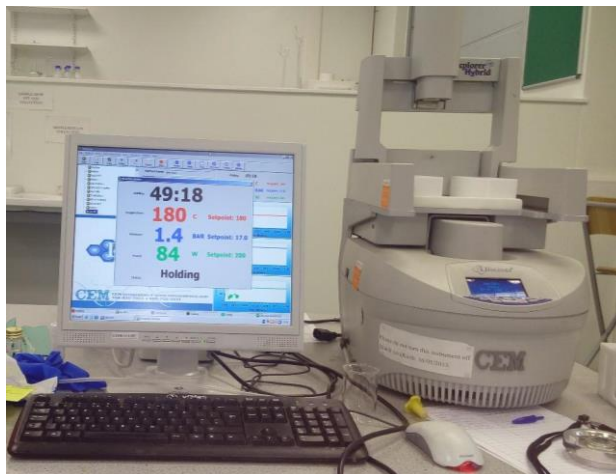
Figure 2.8 PGS synthesis in CEM Discover SP microwave reactor.
