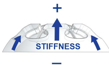
Figure 6.3 Dome shaped scaffold with stiffness gradient, softer in the base and stiffer in the centre.
