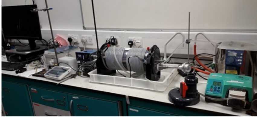
Figure 2.4. Experimental set-up of the home-made SSBR with coiled tubing and process monitoring components
