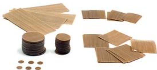
Figure 2.29: PTFE separation foils used to encase the sample within the MeltPrep VCM tool to prevent any sample material sticking to the chamber walls and thus allowing for easy sample removal. ©MeltPrep GmbH
