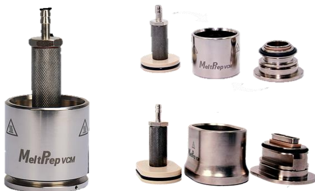
Figure 2.27: Photographs of the 25 mm diameter VCM tool (left and top) supplied with the MeltPrep apparatus consisting of a lid, outer jacket and VCM chamber. The bottom image shows the 10 mm x 40 mm bar tool. ©MeltPrep GmbH
