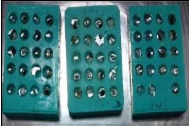
Figure 5: Enamel slabs in silicon moulds
