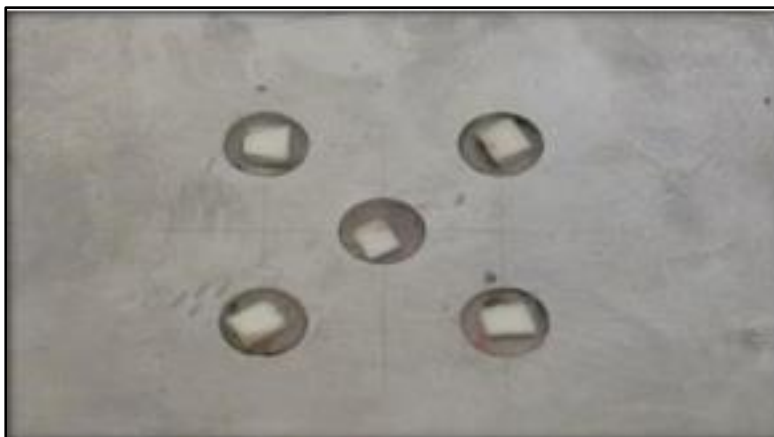
Figure 6: Rectangular steel block holding prepared slabs
