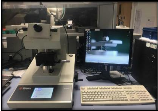
Figure 7: Computer-aided Duramin Indenter Machine (Struers A/S, DK 26- 10, Denmark)
