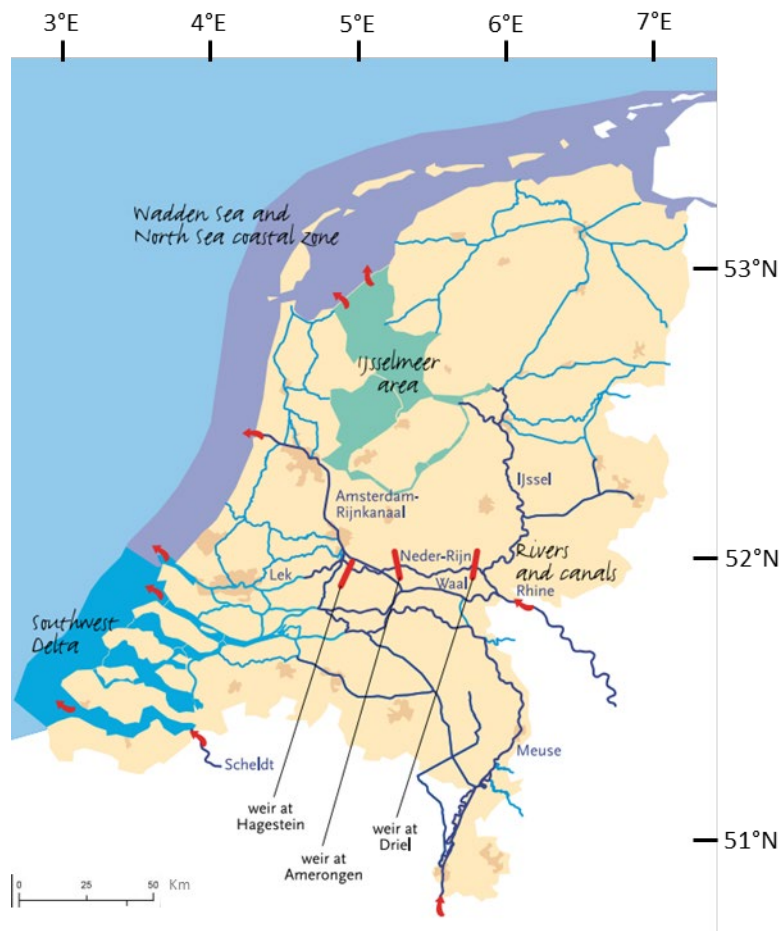
Figure 9 Lay-out of the water management system in the Netherlands, here divided into five major areas: the main rivers (Rhine and Meuse) and associated canals and water control structures (weirs); the IJsselmeer area, an artificial lake created in the 1930s; the southwest Delta with fully closed, semi-closed and open river arms; the closed coastal zone along the North Sea and the tidal mudflat areas of the Wadden Sea in the north; and the “high grounds” areas with small waterways. Source: Rijkswaterstaat (undated)
