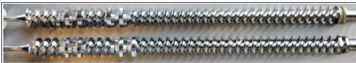
Figure 113: Screw configuration used in this stud which consisted of long pitch conveying elements and two kneading zones each contain 6 kneading discs placed at an angle of 60 degree so a total of 12 kneading discs in each screw.
