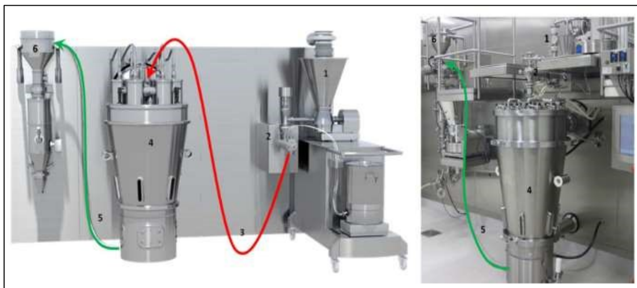
Figure 22: Illustration of the two ConsiGma™-25 (left) Horizontal set-up and (right) vertical setup with the red line represents the wet transfer line (only in horizontal set-up) and the green represents the dry transfer line.
