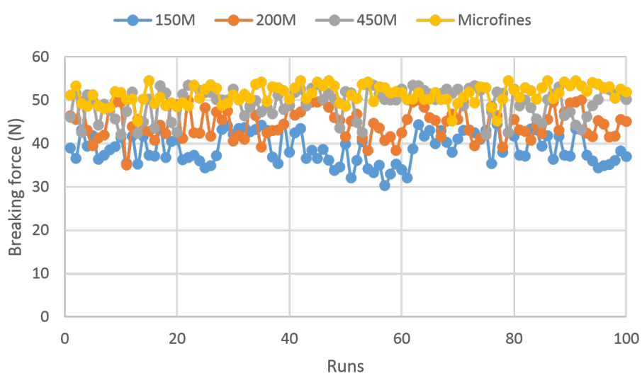
Figure 122: Breaking force variation for 100 tablets of each condition made of different lactose primary particle size (150M, 200M, 450M and microfine). All other parameters during granulation and drying kept fixed throughout i.e., water as a liquid binder, L/S of 0.1, 2 kneading zones, screw speed of 250rpm and drying air temperature, flow rates and drying time of 50°C, 400 m 3 /hr and 800 seconds respectively. The compression force used for tableting was 5kN for all experiment.
