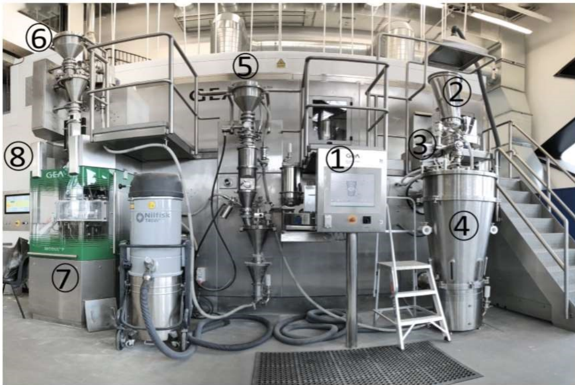
Figure 47: ConsiGma-25 Powder to Tablet line used in this project containing an integrated co-rotating twin screw granulator, six- segmented fluidized bed dryer, milling, formulation and tableting units.
