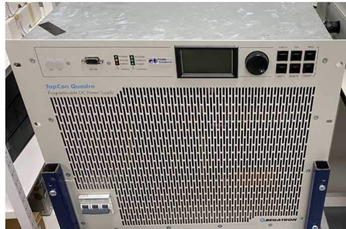
Figure 6.14 1000V DC power supply
