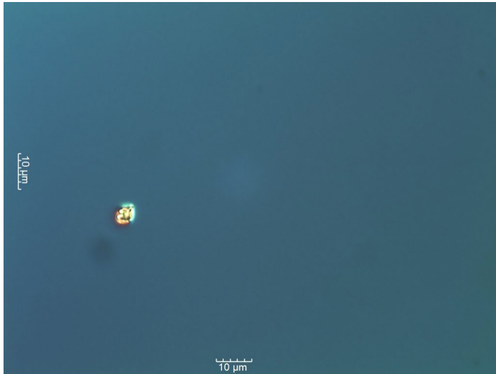
Figure 5.4 Nomarski image of STJ4A 400nm GaAsBi n-i-p (>0.1% Bi) at 50× magnification
