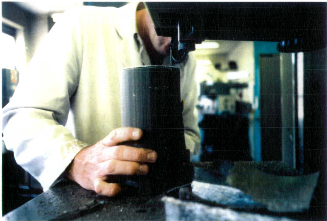
Figure 5.23 - Final stages of block sample trimming showing precision to which specimen may be formed
