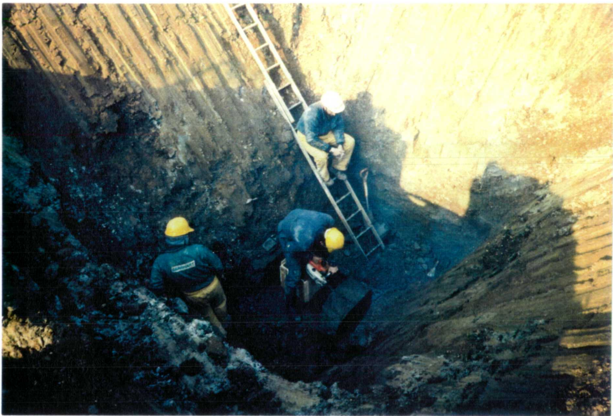
Figure 3.24 - Block sampling in a trial pit at the Elstow excavation
