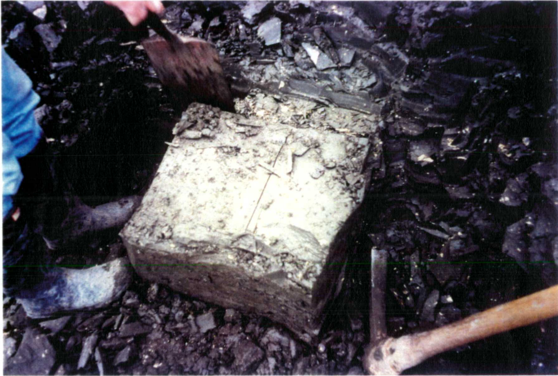
Figure 5.2 - Preparing slope and digging block sample clear of slope
