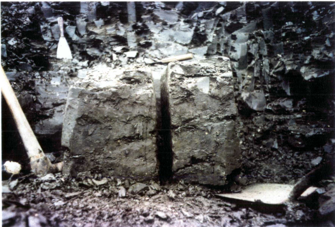
Figure 5.3 - Splitting of block sample into two before sealing and transporting back to the laboratory
