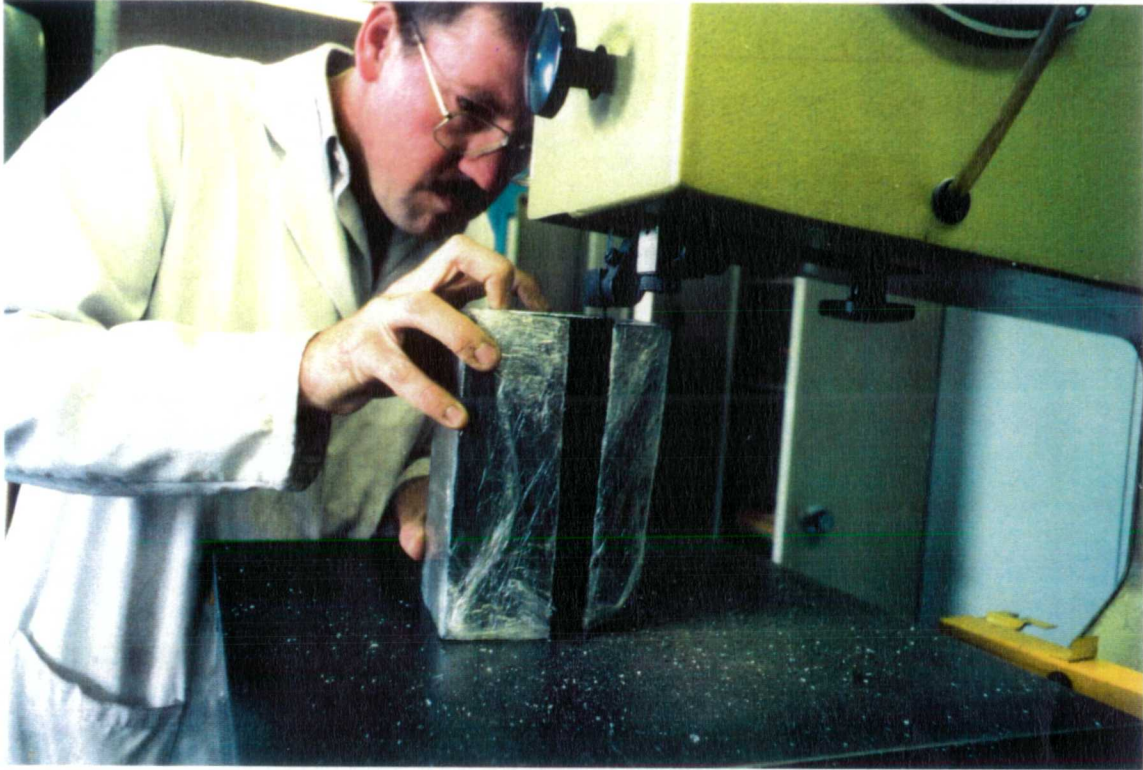
Figure 5.22 - Initial stages of trimming previously sealed block sample section
