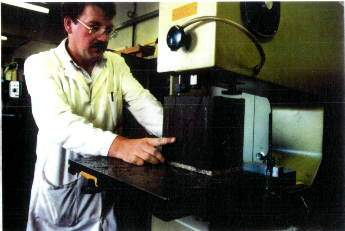
Figure 5.21 - Initial stage of band saw technique involved splitting the soil into manageable sections which could be sealed and stored easily
