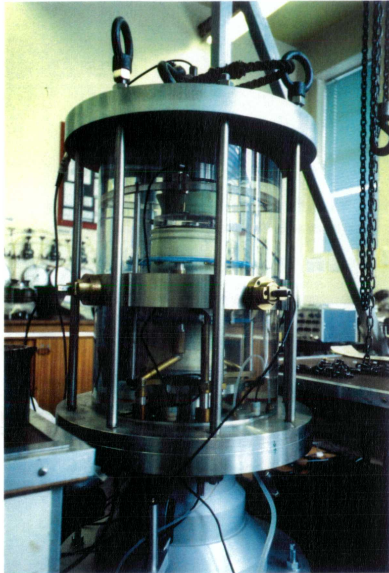
Figure 5.8 - Stress path cell, Cell 2, during a test
