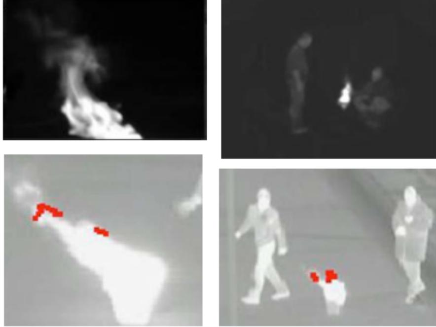
Figure 2.20: Fire images captured by long wavelength microbolometer IR detector (7-14 $\mu\text{m}$ ) [80], [81], [53].(The red highlights were post-processed in the reference, not the original captured image.)
