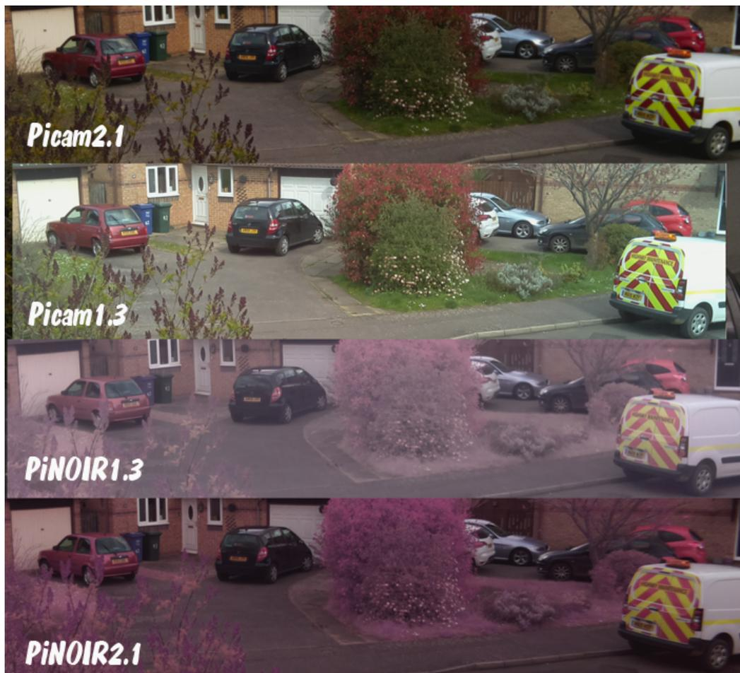
Figure 3.7: From top to bottom: V2, visible; V1, visible, V1, visible+NIR; V2, visible+NIR [129].
