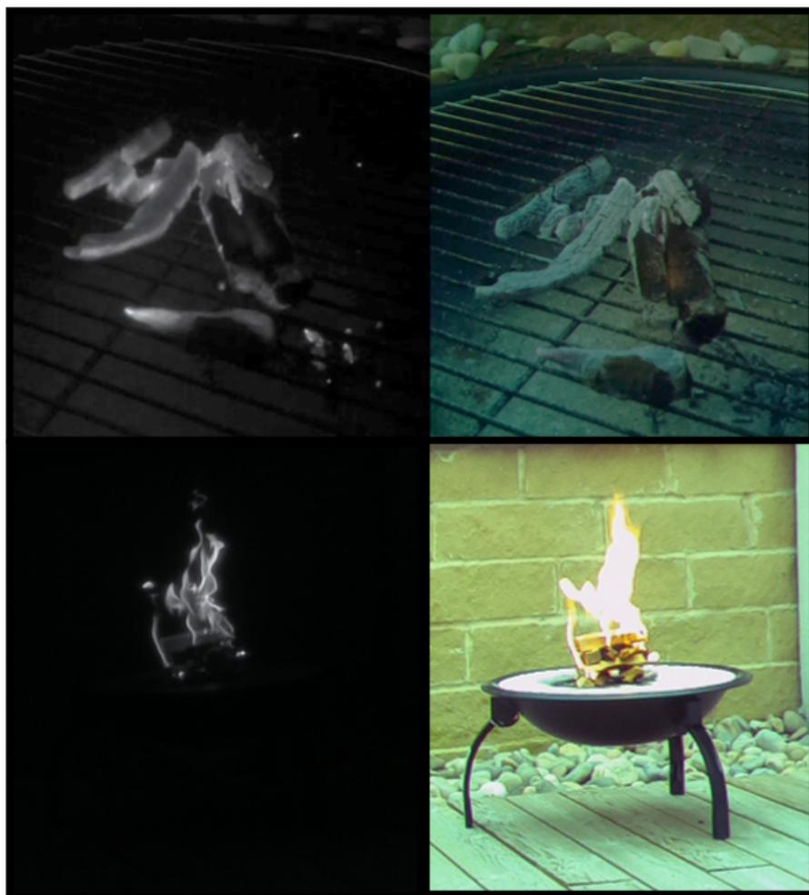
Figure 3.13: NIR and visible image comparisons: smouldering charcoals and a flame. Left: NIR image; Right: visible light image. The flame images were captured on a cloudy day. A cut-on filter at 950 nm was applied to the NIR sensor.
