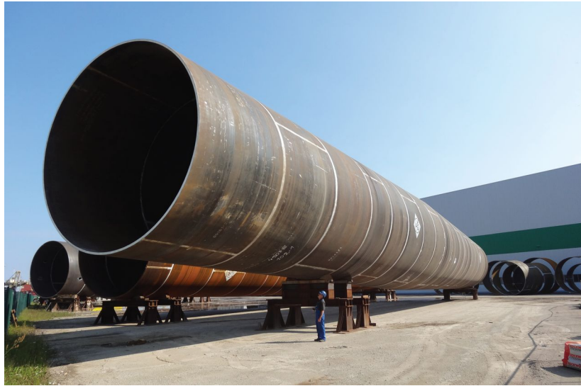
Figure 1.2: Image of monopile leaving production. Credit: Ørsted
