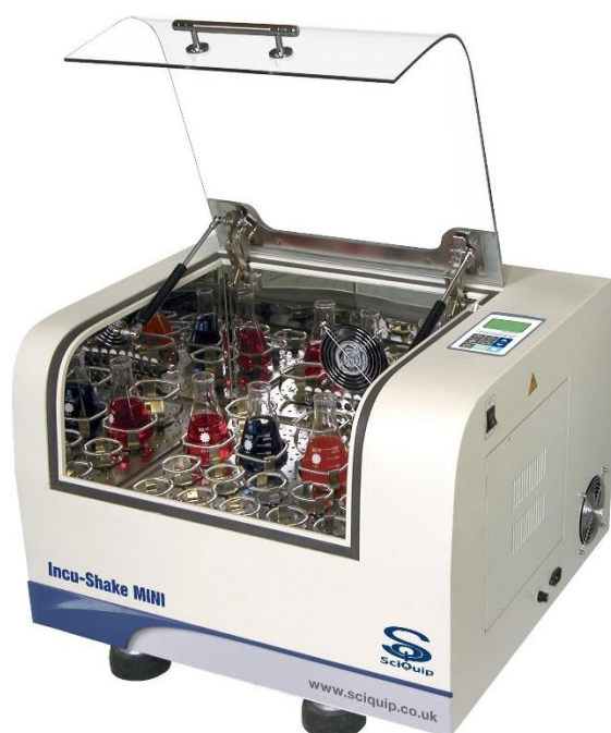
Figure 143 – SciQuip MIDI incubator shaker, the 50mL falcon tube platform was used instead of conical flask holders for reactions. Temperature was set to 37 °C and a shaker speed of 500 rpm. The unit was pre-heated for 15 minutes before use.
