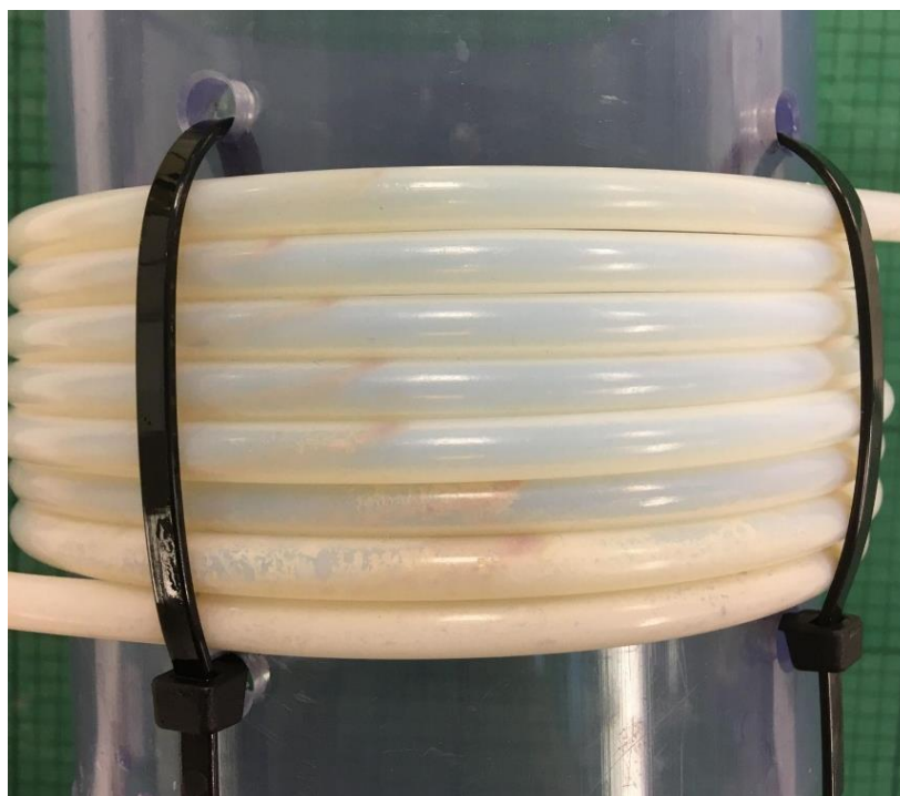
Figure 94 – Fouling residue observed in the 300 cm (4.5 mm ID) reactor (Table 12, Entry 8).
