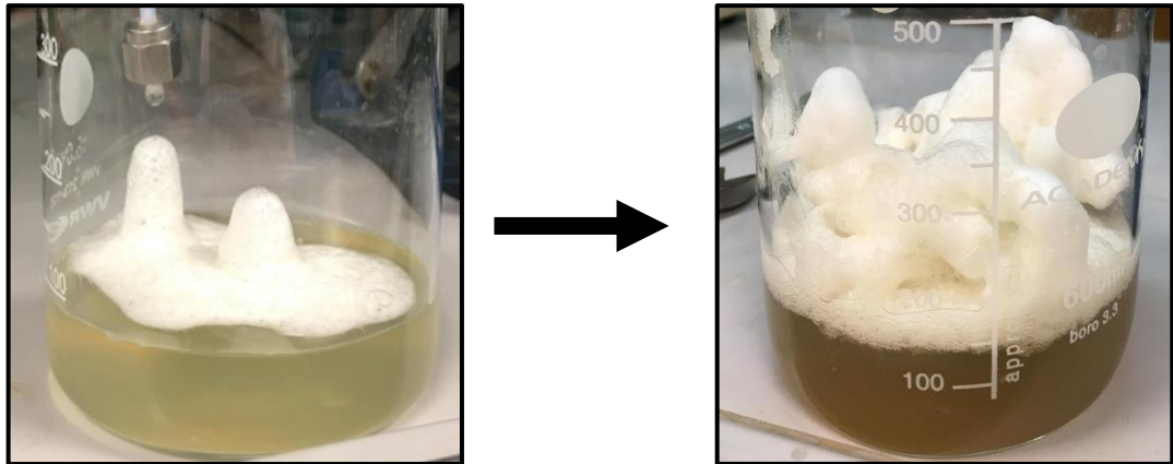
Figure 87 – Foam “stalagmites” formed from the continual dripping of solution and foam out of the reactor, demonstrating the foams excellent stability.
