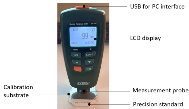
Figure 2-18. A photograph of the Extech™ Coating Thickness tester CG204 device showing calibration with a 99μm standard (Photograph taken by author).
