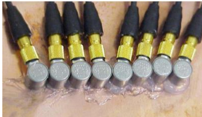
Figure 4-7. A photograph showing eight 5MHz planar piston contact transducers closely spaced that were coupled on to a copper block with coupling gel (extracted from [7]). Each contact transducer is 12.7mm in diameter.
