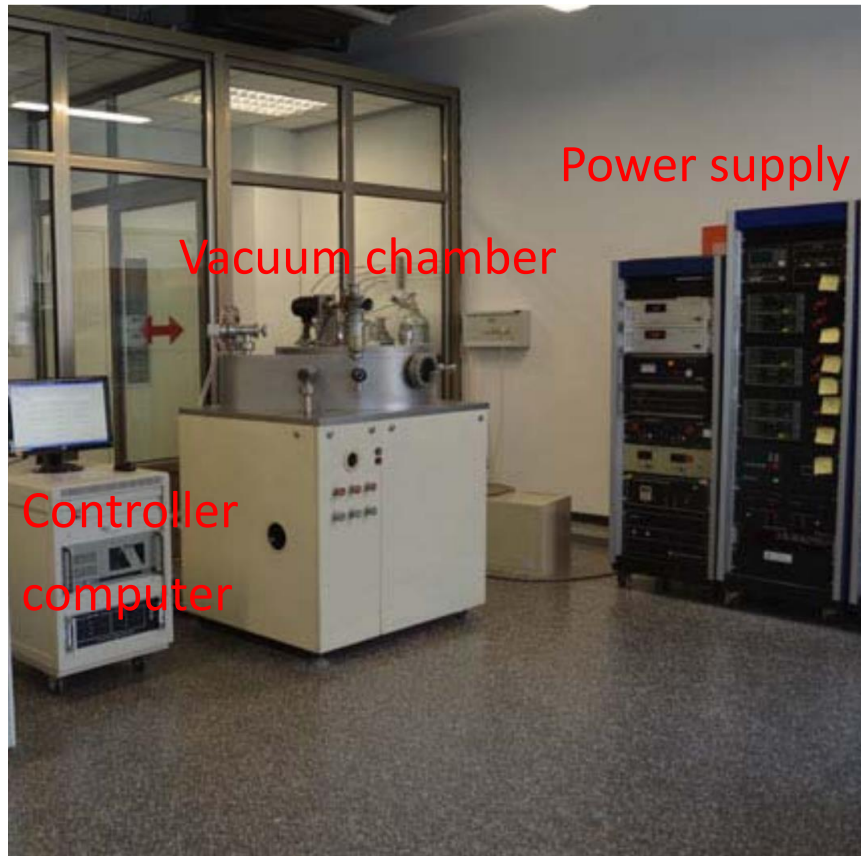
Figure 3.2 The magnetron sputtering instrument used in this thesis. The red notes exhibit the different components of magnetron sputtering, including power supply (DC power and RF power), vacuum chamber and controller computer.
