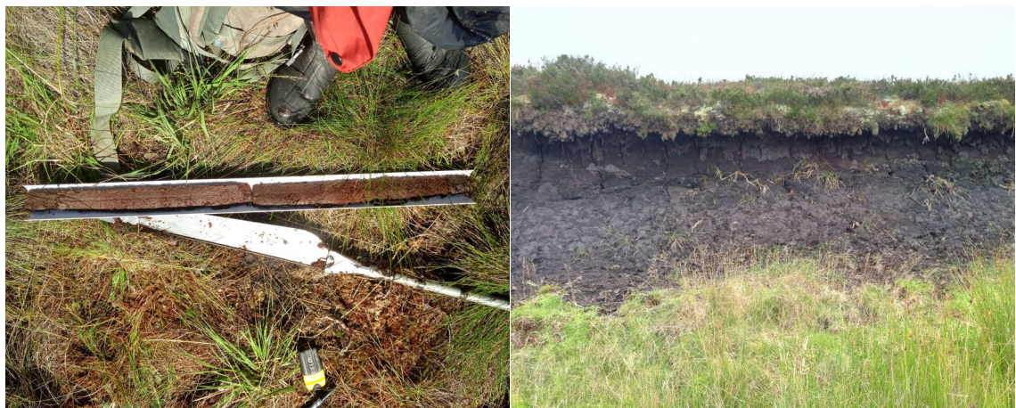
Figure 1-4 – Fresh peat taken from Flanders Moss West (left) and exposed dried, cracked peat at Talaheel, Flow Country (right).
