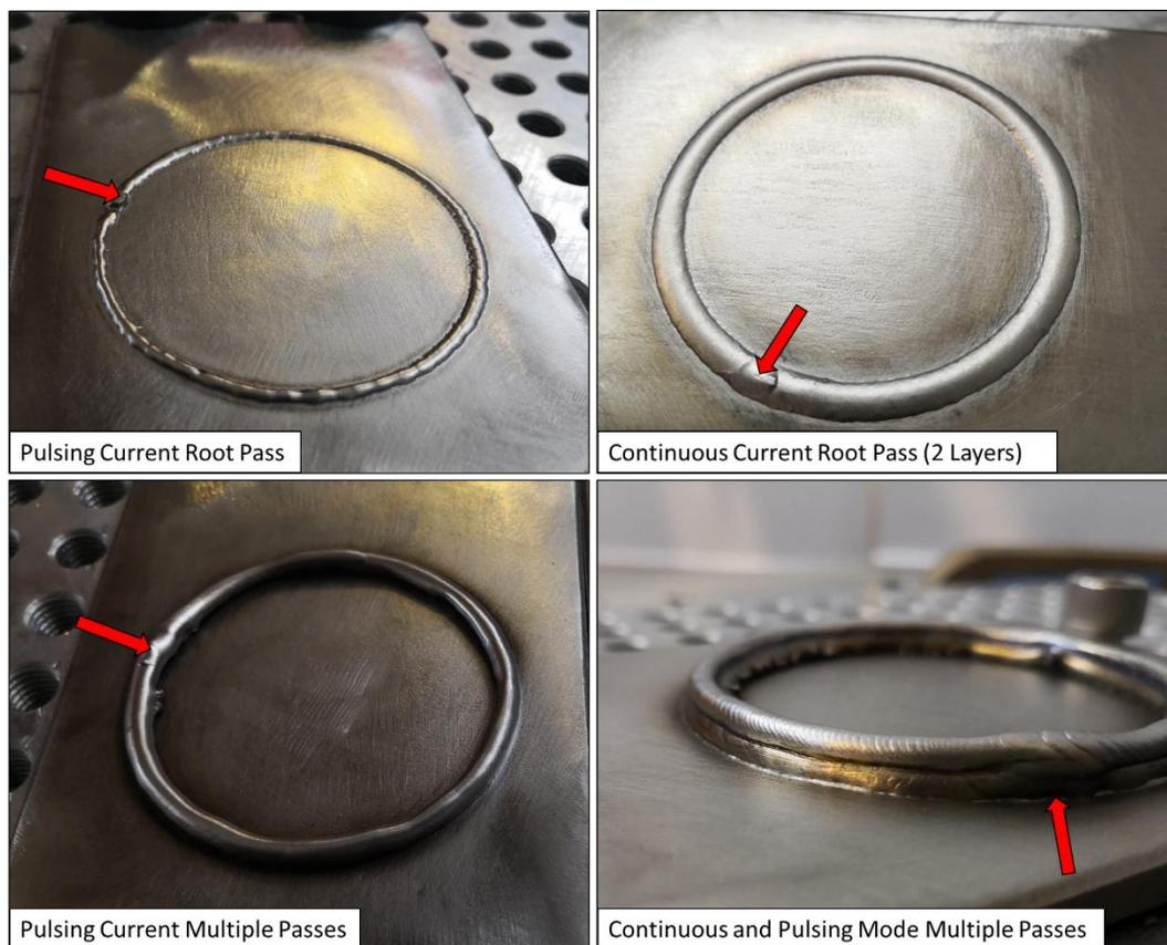
Figure 4.25 – Circular root and built-up passes on wire arc additive manufacturing. The arrows mark the starting/ending point where passes overlap.
