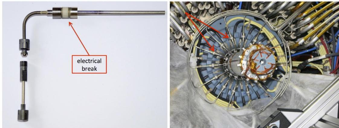
Figure 2.10 – Left: Titanium fitting and electrical break developed for the Insertable B-Layer (IBL). Right: Electrical breaks in situ at the ends of the IBL staves [13].
