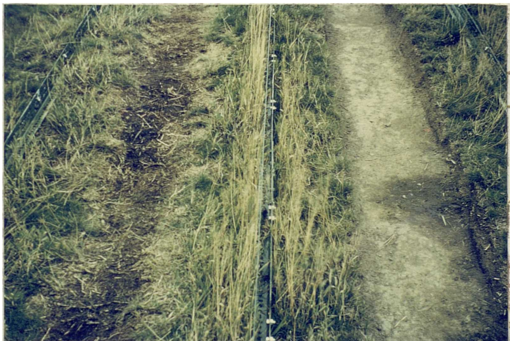
PLATE 10 Angle iron framework from which profile changes were measured on the Bradfield paths
