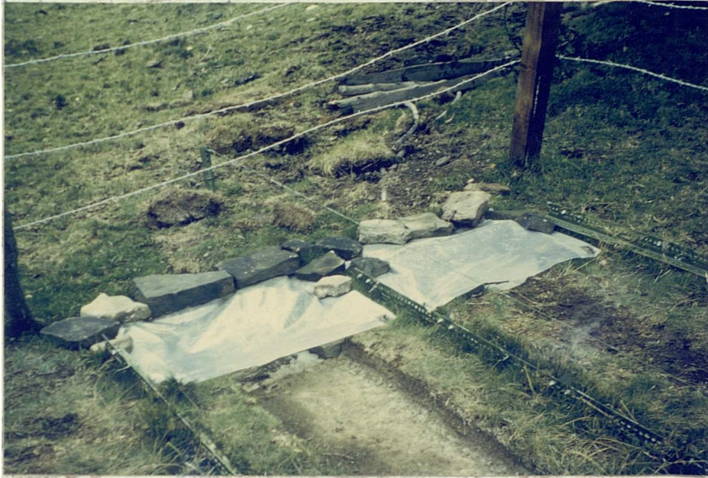
PLATE 9 Covered troughs to collect water and sediment from the Bradfield paths
