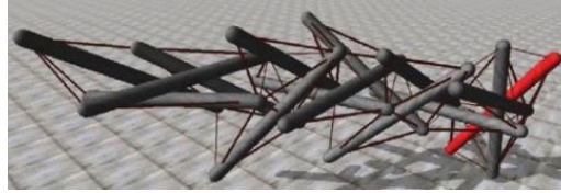
Figure 2.21 The 15-strut tensegrity structure model included high degrees of dynamic linkages[38, 39].
