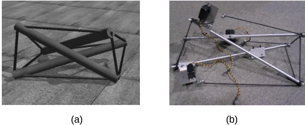
Figure 2.4 TR-3 design [36]: (a) TR-3 simulation model; and (b) TR-3 prototype.
