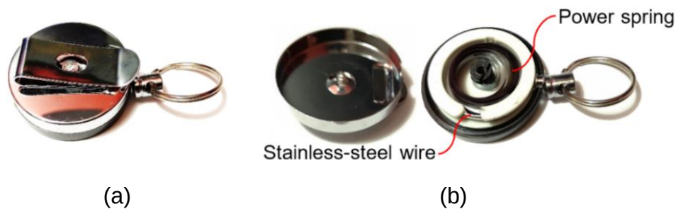
Figure 4.19 Images of the retractable key chain (RC): (a) assembled case (original item) and (b) disassembled case.
