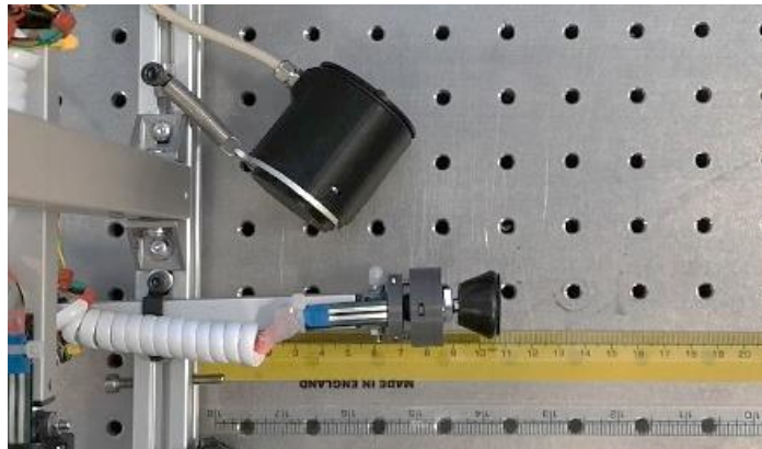
Figure 5.29 The experimental setup of the locking and unlocking delay time.
