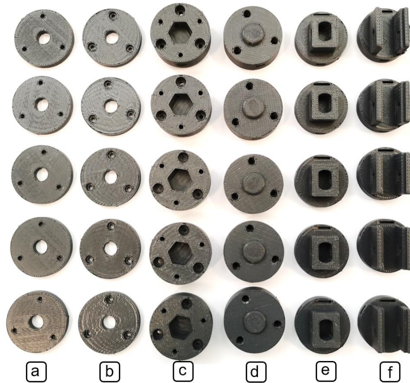
Figure A-1 Image of end cap parts (five sets) created from 3D printing technology: (a) ball joint holder of the linear actuator (LA) base tip, (b) ball joint holder of the Slider tip, (c) pressing plate of the LA-base tip, (d) pressing plate of the slider tip, (e) the connecting base of the slider tip and (f) the connecting base of the LA base tip.
