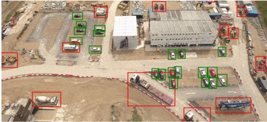
Drone imagery showing object detection using artificial intelligence (Kaila, 2018).
