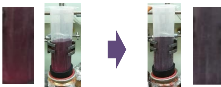
Figure 5.9 The appearance of Amberlite XAD-7HP resin on the left after elution with acidified wash (red) and on the right after elution with a copious amount of water (bluish-red).
