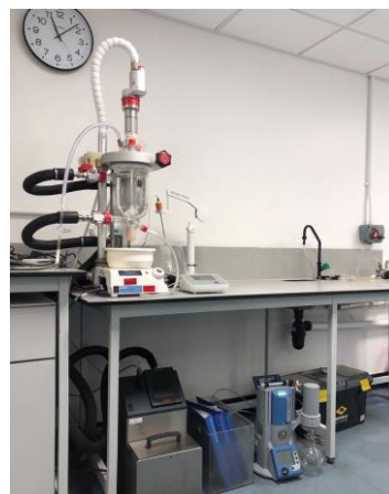
Figure 4-16 Sketch diagram (left) and equipment (right) of experimental setup for autoreactor synthesised C-S-H.
