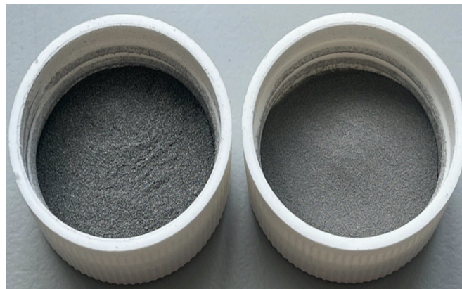
Figure 8: HDH powders (left side) and GA powders (right side).
