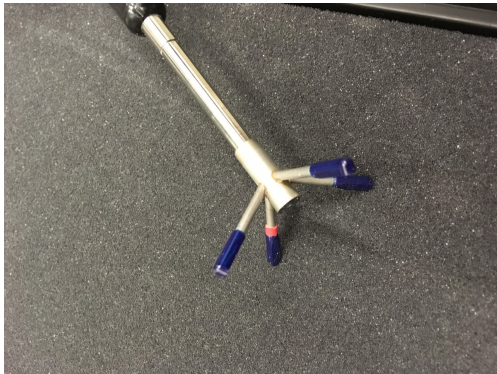
(a) Nortek Vectrino II ADV sensor used in the experiments.
