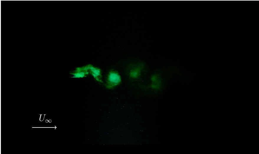
Figure 6.11: Dye flow visualisation of the circular cylinder wake at Re_D = 2100 .
