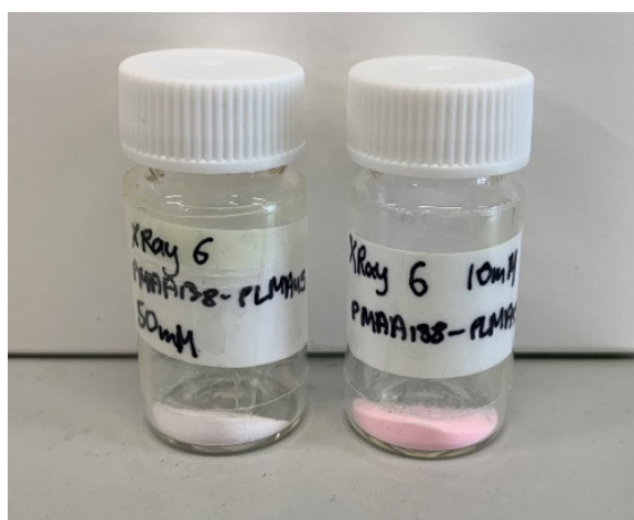
Figure 42. LHS: Calcite crystals collected after crystallisation using 50 mM [Ca^{2+}] , 11.9 mg PMAA 138 -PLMA 45 and X-RAY 6 as the oil phase. White appearance indicates unsuccessful occlusion. RHS: Calcite crystals collected after crystallisation using 10 mM [Ca^{2+}] , 11.9 mg PMAA 138 -PLMA 45 and X-RAY 6 as the oil phase. The pink hue indicates successful oil occlusion within these crystals.
