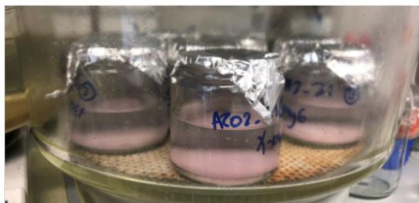
Figure 39. Gravitational sedimentation of pink calcite crystals observed after 24 h when using the ammonia diffusion method at 50 mM \text{CaCl}_2 . The pink colouration arises from the presence of Nile Red dye dissolved in the oil phase (methyl myristate in this case).
