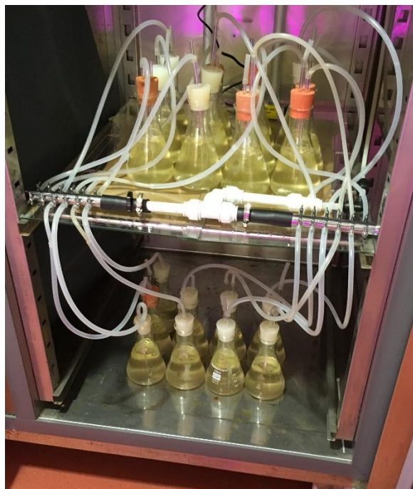
Figure 4.9 - Experimental setup for high throughput screening of culture condition optimisation for biorefining. Cultures contained 200 mL of liquid volume and were aerated with a sterile gas mixture of air and 0.5 % CO 2
