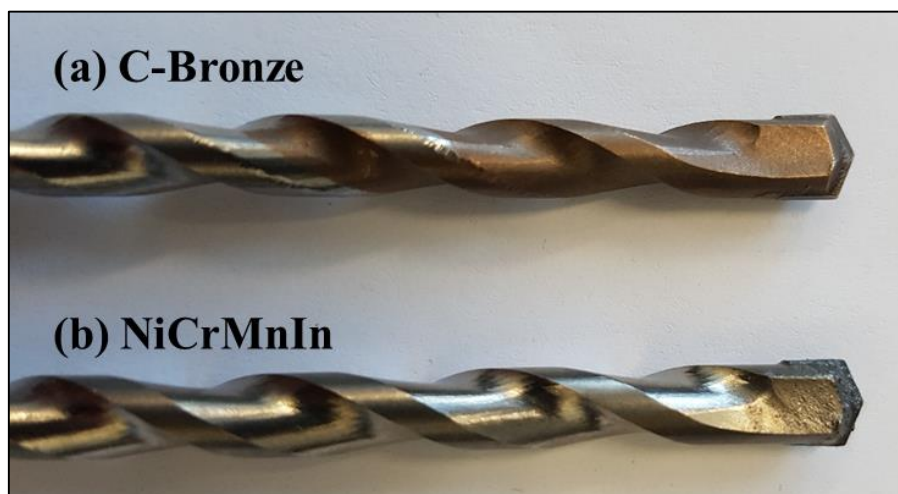
Figure 10.17: Photograph taken of example drill bits brazed using (a) commercial C-Bronze filler metal and (b) optimised NiCrMnIn filler metal.
