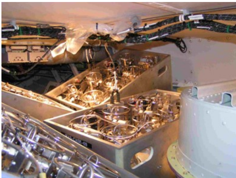
Figure 2.3: Cases for the WAS system in the rear hold of the FAAM aircraft.
