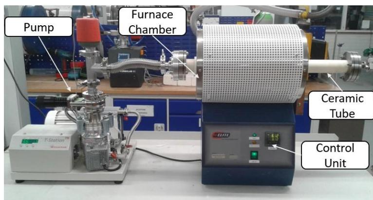
**Figure 2.13:** An image of the diffusion couple rig used for the diffusion couple experiment.
