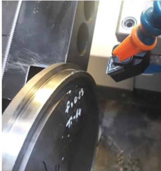
**Figure 3.5:** Photograph showing the setup for the industrial machining trials. Using a disk of material held inside a CNC machining centre; the cutting insert held into a dynamometer to record the cutting forces and the coolant provided through an external pipe.
