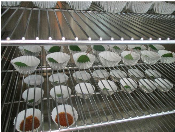
Figure 11. Determining leaf relative water content ( RWC_L ). It requires the rehydration of sampled leaves (top left) after obtaining their fresh weight (top right). Samples are then closed in a box to rehydrate overnight and re-weighed in the morning. Leaves are then left to dry in a drying cabinet for 24 h at 70 °C (bottom left), after which samples are weighed again for dry weight (bottom right) and for the calculation of RWC_L .
