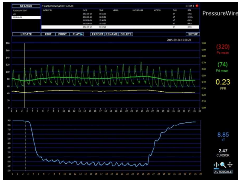
Figure 5.5: Thermodilution protocol- part 1. Pressure wire placed within guiding catheter to record the temperature of the infusate (Ti). There was no simultaneous distal pressure recording as the manifold setup did not allow that when infusing saline. Therefore, the Pa value and FFR value are erroneous.
