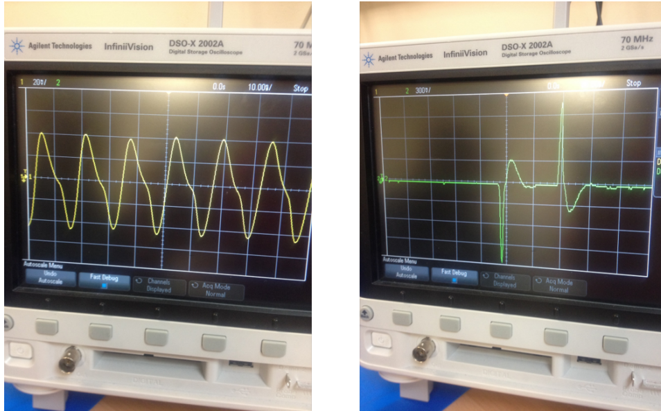
Figure A.1: Oscilloscope measurements of the (a) sync pulse and (b) trigger pulse
