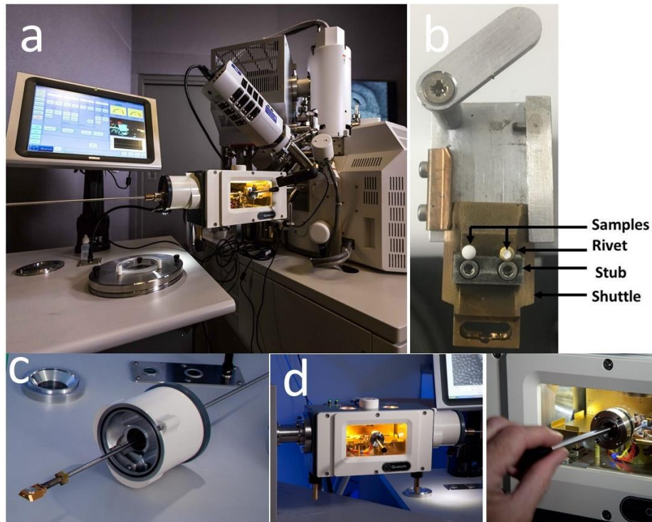
Figure 3-16. Digital images of (a) Cryo-SEM system (b) samples were pipetted on the rivets, which was attached with a shuttle (c) The cryo transfer device with shuttle and rivets (d) a cryo preparation chamber (Quilo) and (e) Twin fracturing tools manipulators.
